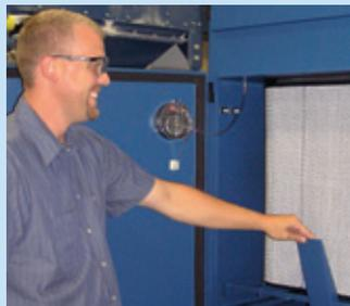
*One pivot lever securely retains the primary filter element*
