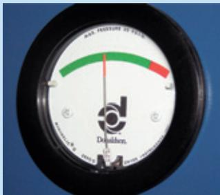
*Differential pressure gauge(s) identifies filter maintenance*
